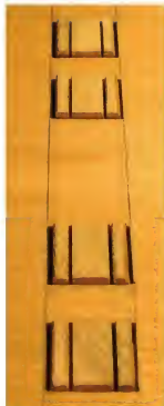
All together now. Dry assemble the joint, and take a deep breath before glue-up.
